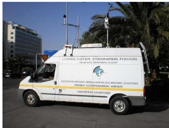
Figure 6: Noise measurements with the IERSD mobile station.
